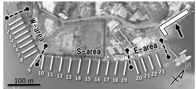
Fig. 2. Arrangement of survey lines with the bottom topography along the stone-built seawall mound at the study site. Arrow shows the new seawall mound after first survey in this study.
